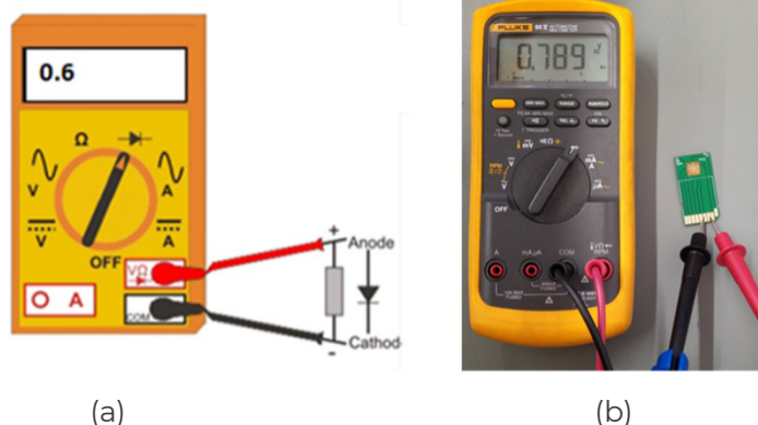
Figure 4. (a) Connection of the multimeter with the parallel resistor. (b) Image of a real measure without parallel resistor.
