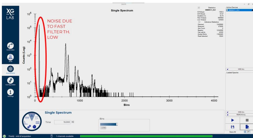
Figure 6: With the “Zero Peak rate = 0” a peak at bin 96 is due to noise
