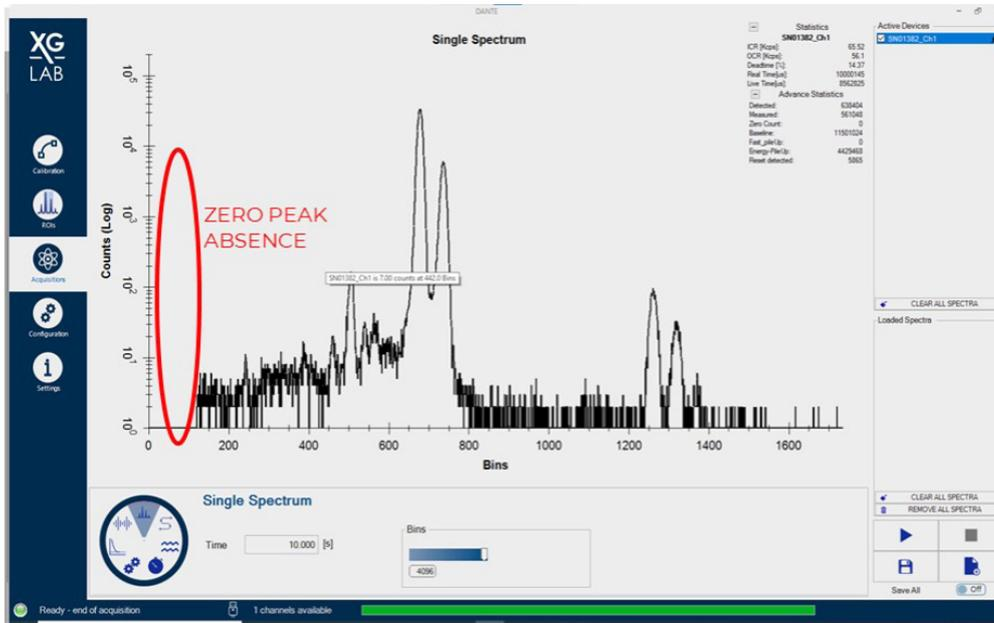
Figure 7: Zero Peak disabled and correct Fast Filter Threshold setting
