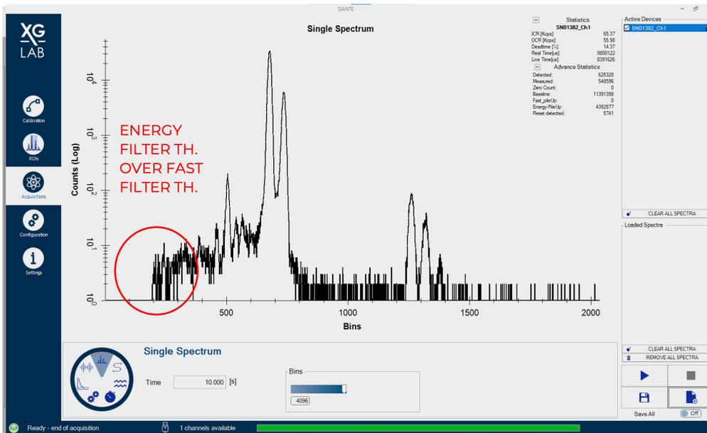
Figure 8: Incorrect use of Energy Filter threshold
