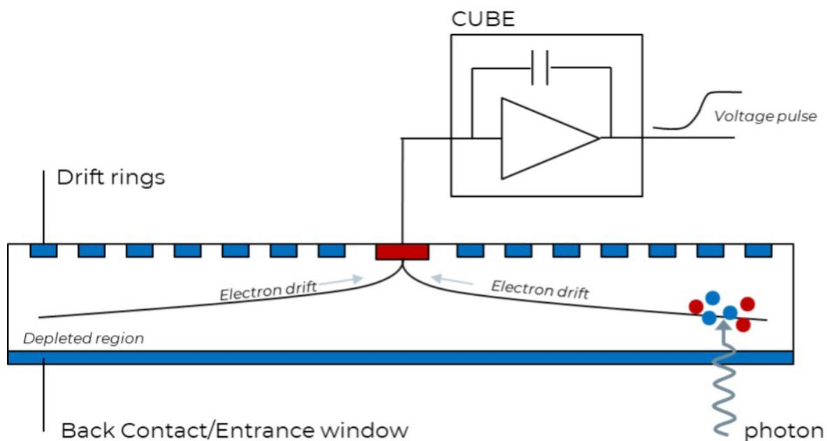
Figure 1. SDD cross-section and working principle
