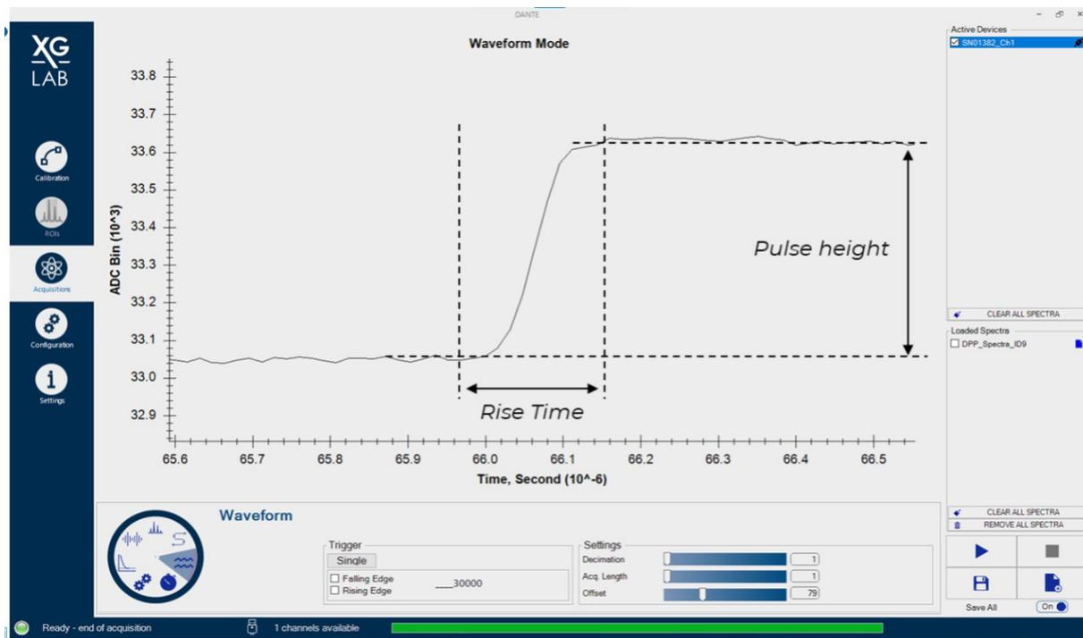
Figure 3: Pulse signal, corresponding to the detection of one photon, acquired by DANTE at the output of a CUBE preamplifier connected to an SDD.
