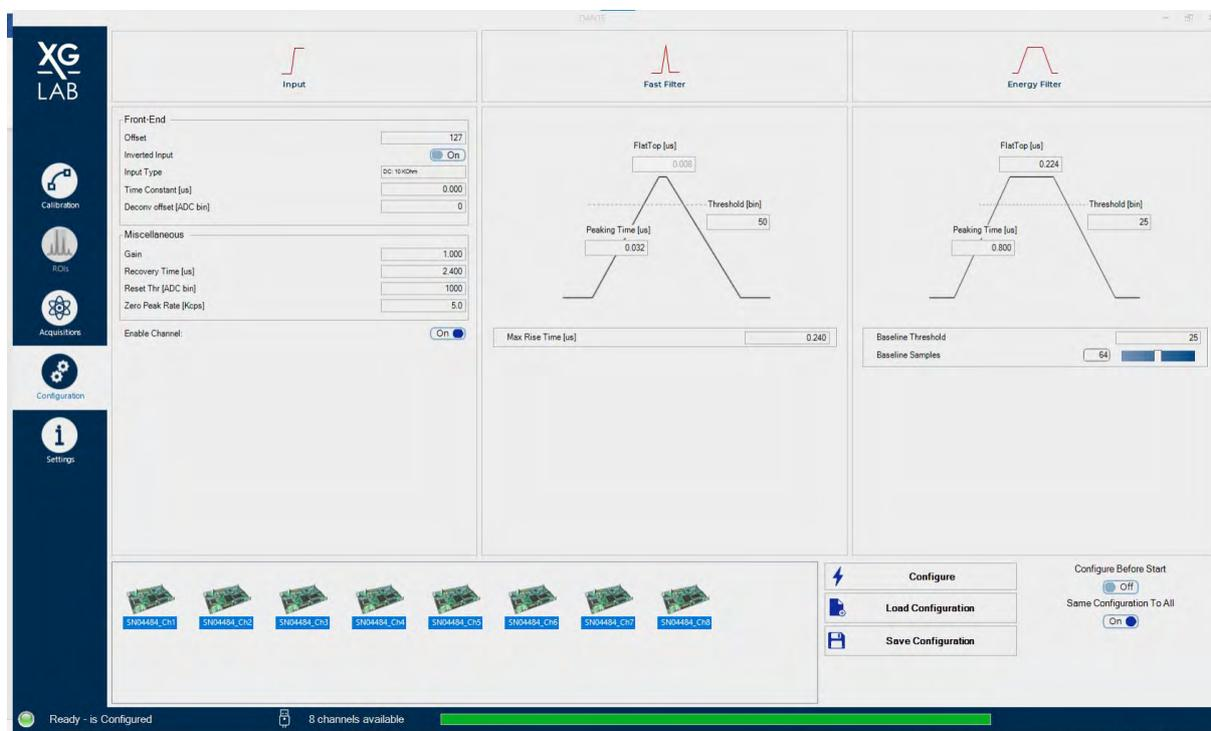
Figure 2: Configuration Window in the DANTE acquisition software
