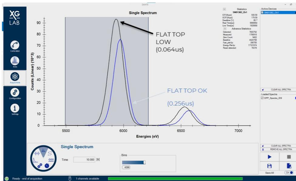
Figure 11: Ballistic deficit produced by low Flat Top value
