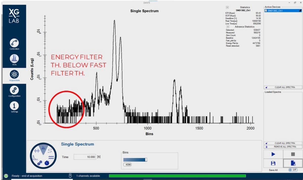
Figure 9: Proper use of Energy Filter threshold. Low energy events are correctly measured
