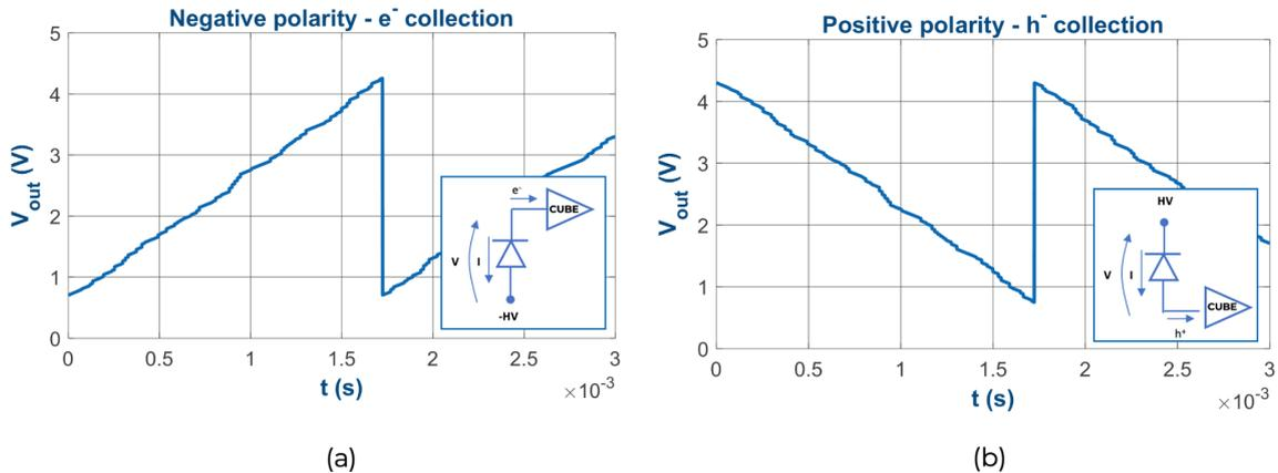
Figure 2. CUBE amplifier output in case of (a) electrons collection or (b) holes collection
