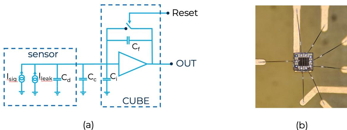
Figure 1. (a) Electrical schematic of the CUBE preamplifier connected to a generic sensor; (b) a CUBE PRE033 glued, and wire bonded to a board.
