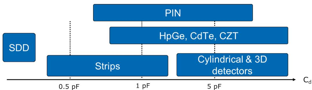
Figure 3. Input capacitance ranges for different radiation detector types
