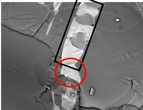
BSED image obtained using a state-of-the-art annular 4-segment solid-state detector in which the segments are arranged under the pole piece of the SEM
