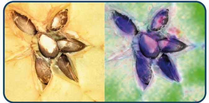
Apple Core Slice Mapping of Ca (blue), K (green) and S (red)
